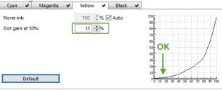
o Note that increasing the dot gain may increase the light ink usage and overall ink consumption significantly!
