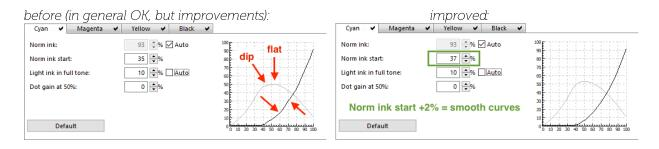
If no improvement can be made regardless of the settings used, re-print and re-measure the linearization charts and/or check the performance of your measuring device.
