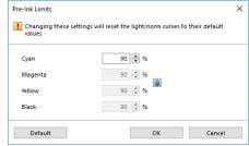
Note that some printers support a custom pre-linearization which is applied in the background when printing the linearization charts. The pre-linearization is valid only for the default pre-ink-limit it was created for. Any change in the pre-ink-limit results in the linearization charts being printed without the pre-linearization.
