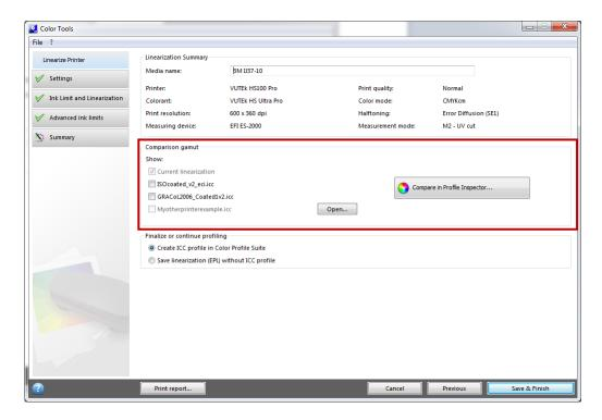
It allows you to evaluate or compare the gamut of your linearization with one of the standard reference color spaces and/or any custom ICC profile. Click "Compare in Profiler Inspector" to start Fiery Profile Inspector:
