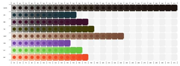
The top edge contains the column headings, representing the TIL level of a given column. The TIL levels increase left-to-right from the "Range start" value (default: 50%) to the "Range end" value (default: maximum possible ink; e.g.: 313%) in a defined step size (e.g. 10%).
