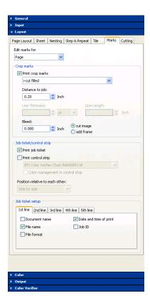
The crop marks define the position of the substrate on the table and are automatically placed around the image for which they have been selected. You can adjust the position of all crop marks in relation to the image by editing the bleed value on the Marks tab. However, it is not possible to add, delete or change the position of individual marks.
