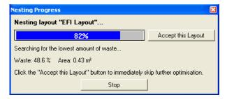
During the search, a dialog shows the progress indicator, the current waste percentage and the area. The Waste is the surface outside the cut paths in % of the total surface, and the area is the surface of the bounding box of all cut paths.
