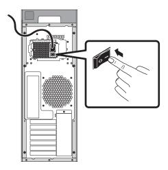
**FIGURE 1:** Fiery proServer power switch
