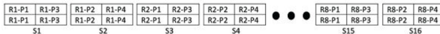
Figure 4: Example of single-record imposition using Repeat-Collate Cut for 8 records, 4 pages per record, 2 rows x 2 columns layout, 1 row x 2 columns product, simplex. R = Record, P = Page, S = Sheet.
