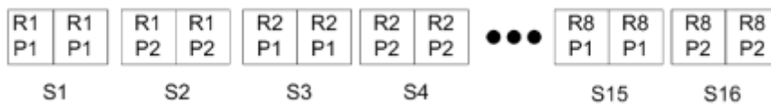
Figure 2: Example of single-record imposition using Unique Gangup for 8 records, 2 pages per record, 1 row x 2 columns layout, simplex. R = Record, P = Page, S = Sheet.
