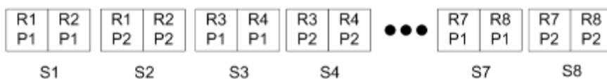
Figure 4: Example of Multi-Record Collate for 8 records, 2 pages per record, 1 row x 2 columns layout, simplex. R = Record, P = Page, S = Sheet
